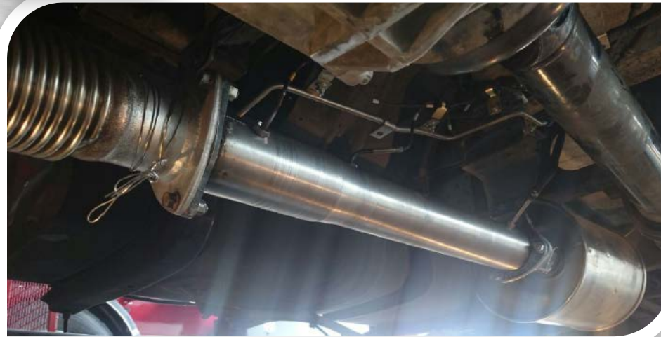
Replaced pipe instead of DOC/DPF muffler
